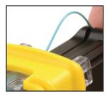
**Maximum Reliability** — Bow feature maintains proper pressure of fiber ends to eliminate air gaps during termination
