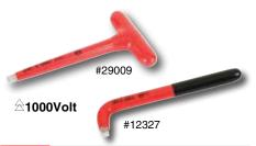
1000Volt Insulated 3/8" Drive T-handle Or Breaker Bar. Insulation according to EN/IEC 60900 specification, up to 1000Volt Rated. Individually Tested. Blade chromevanadium steel, hardened.
