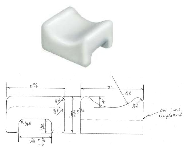
TOLERANCE UNLESS OTHERWISE SPEC. ±.015 PER INCH ON DIM. OF ONE INCH OR MORE, BUT NOT LESS THAN ±.015.
