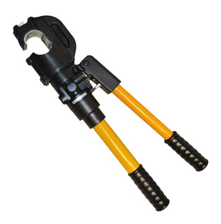
The **EP-430** is unique in that it has a large jaw opening of 1-3/16" and is able to splice up to 600 MCM. This tool was designed for the electrical contractor or electric utility lineman who is confronted with larger cable diameters and larger connectors. Similar competitive tools are limited to a .95" jaw opening that drastically reduces their connecting range. Most internal hydraulic components are the same as the EP-410 and EP-510.
