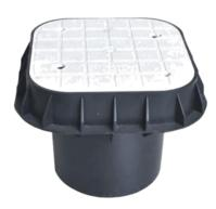
The light duty earth inspection housing has a maximum safe working load of 5,000 kgs. It is UV stabilized against degradation by sunlight and non-brittle to prevent cold weather damage, The unique, detachable easy-locking lid ensures security of equipment as the locking mechanism can only be operated by the special key provided with the housing,
